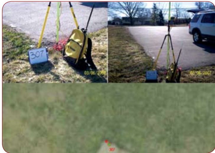
Fig. 6: Optimal checkpoint location 307. The survey checkpoint (green) and photo identified locations (red) are shown.
