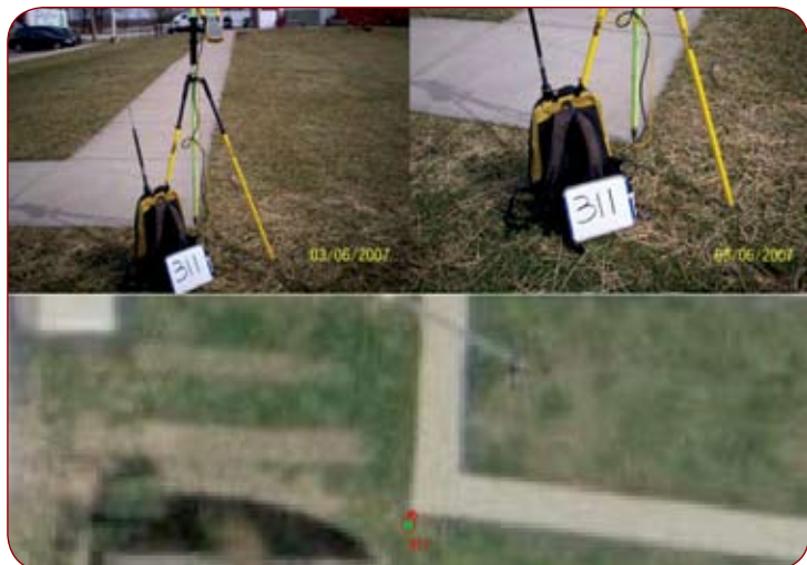
Fig. 7: Optimal checkpoint location 311. The survey checkpoint (green) and photo identified locations (red) are shown.
